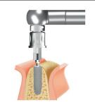
Remove the torque-ratchet wrench [GAN-469-1000203] and pull the screwtool out vertically.
