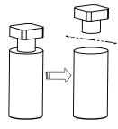
The S-TD250 transfer can be used as a castable sheath for the Slim 2.5 implant abutment.
